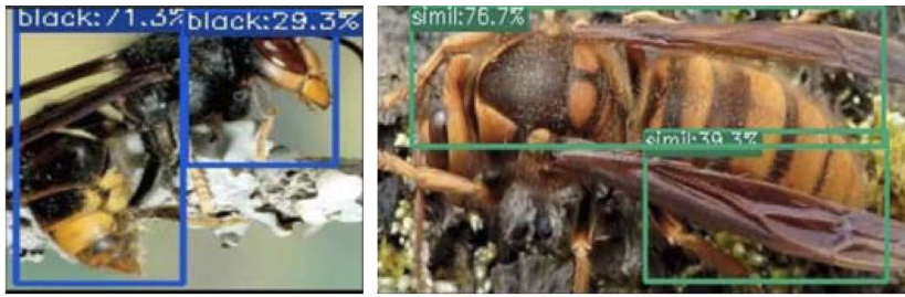
Fig. 15. Examples of detection error, when the size difference between adjacent bounding boxes is large in proposed method.
