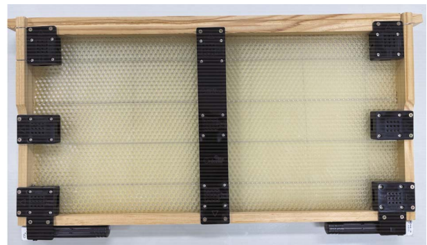
Fig. 1. Temperature sensor installed in the empty comb.
