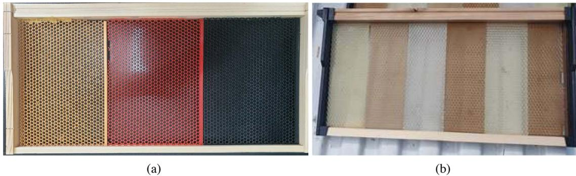
**Fig. 3.** Brood frames assembled with different types of composite combs cut into 1/3 and 1/6 sizes for field testing.
