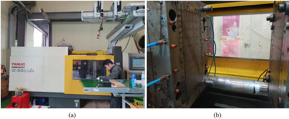
Fig. 2. (a) An electric injection molding machine used in this experiment and (b) molds mounted within it.
